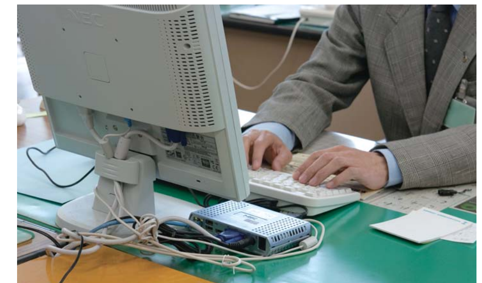
A palm-sized thin client terminal "US110" with a high-speed video/audio processing capability
